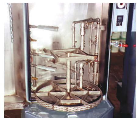
(3) Model 2012 12" (305mm) Standard Air Knives perform the drying cycle in this parts washer.
