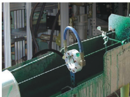
A Model 2431 1" (25mm) Standard Air Wipe blows off the excess coating from a wire into a dip tank.
