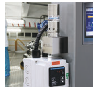
Cabinet Cooler Systems with ETC provide temperature control.
